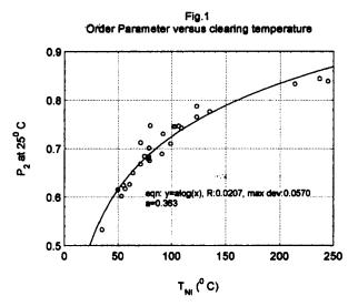
Using this relation, order parameters of arbitrary compounds at  $25^{\circ}$  C can be calculated, when the clearing temperatures  $T_{NI}$  are known. When data for  $T_{NI}$  are lacking, they can be approximately evaluated by the procedure included in the data base "LIQCRYST"<sup>[9]</sup>, or for two ring compounds by the method of Vill<sup>[10]</sup>.
